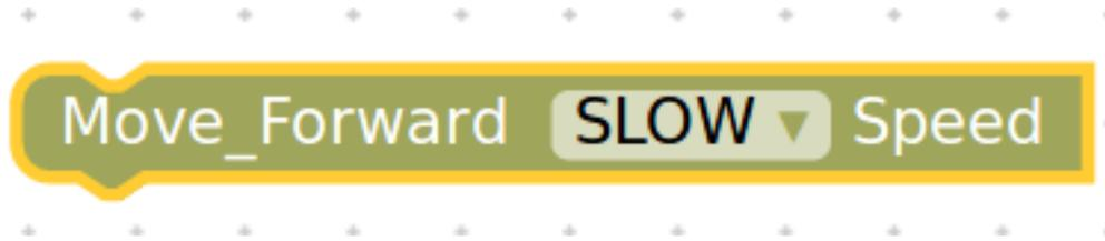
**Move Forward** is a custom block that moves the TurtleBot3 forward in one of three speed modes - SLOW, NORMAL and FAST. A python script called `move_forward.py` shown below is the backend code for this block.
